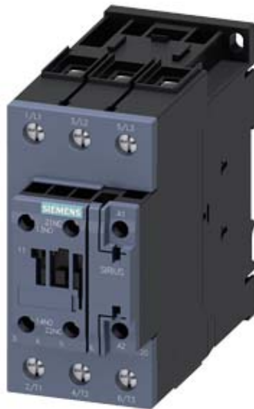
CONTACTOR,AC3:18.5KW/400V, 1NO+1NC, 110V AC 50HZ, 3-POLE, SIZE S2, SCREW TERMINAL
