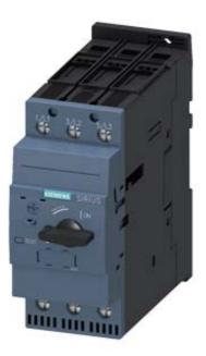
CIRCUIT BREAKER, SIZE S2, FOR MOTOR PROTECTION, CLASS 10, A-RELEASE 14...20A, N-RELEASE 260A, SCREW TERMINAL, INCREASED SWITCHING CAPACITY
