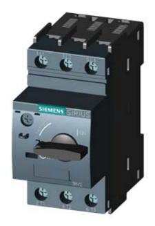
CIRCUIT-BREAKER SZ S00, FOR MOTOR PROTECTION, CLASS 10, A-REL.1.8...2.5A, N-RELEASE 33A, SCREW CONNECTION, STANDARD SW. CAPACITY
